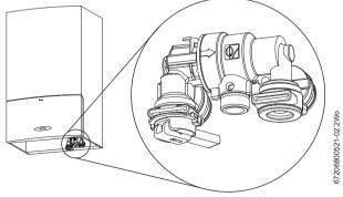
Fig. 3 Integral filling link location
