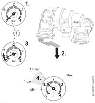
Fig. 4 Keyless filling link
