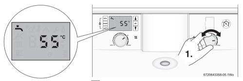
The value is displayed during this process, press obtained to exit or after five seconds of inactivity the boiler display will return to the default screen
