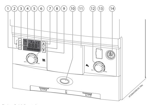
Fig. 1 Basic boiler controls
